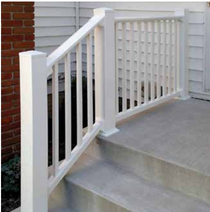
STANDARD BALUSTER 7/8" x 1-1/2" Rectangular Vinyl 2-7/8" Baluster Spacing
