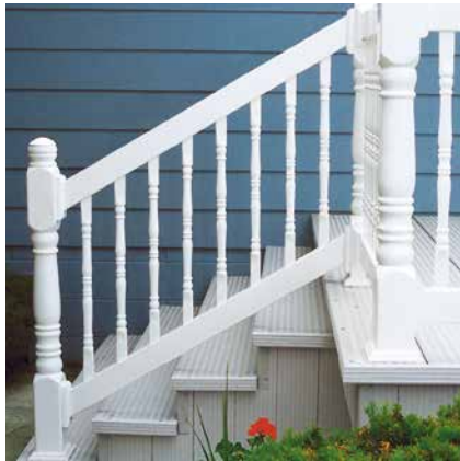
"A" SERIES BALUSTER 7/8" x 1-1/2" Decorative Vinyl 2-7/8" Baluster Spacing 42" Balusters are Aluminum Reinforced
